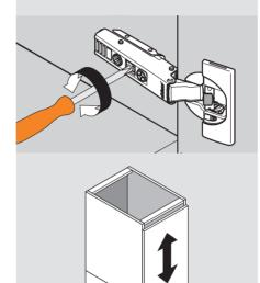
NOTE: On non-cam mounting plates, loosen screws, adjust door and retighten screws
